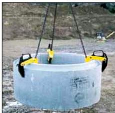
**Load hoisting tackles for underground construction**
