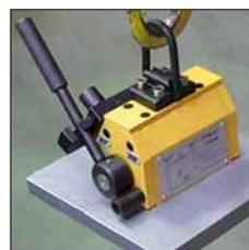
Permanent load lifting magnets
